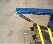
Each corner of the bed has 4 D-Rings. Start by attaching one spring per corner working from corner to corner in a circular motion. Attach the spring on the first D-ring and the first triangle on the frame. This first triangle will also have the quick link attached to it. Once the first springs are in place, go to the second D-ring and attach it to the third triangle on the frame. (You will skip a triangle on the frame)
