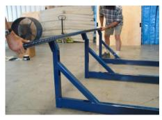
Put the tops on the legs starting and then the tops with the middle leg.
