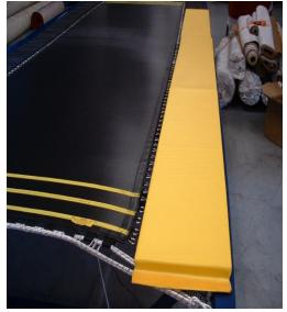
Attach the Velcro along the length of the frame. Your pads will attach to the Velcro and secure them in place.
