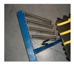
You will skip a spot on the frame for each D-ring spring. Continue to work in the circular motion until the first 4 D-ring springs have been attached on all four corners.
